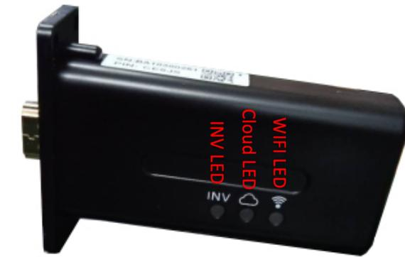
After set password successfully, the Cloud LED of wifi will blink for about 2 minutes, and then it is solid on, which indicate that the wifi module has successfully connected to the wireless network. After 5 minutes, the INV LED of the WiFi module is always on, indicating that the wifi module and the inverter are successfully communicated. After 10 minutes, you can check the information about the system by website or APP.
